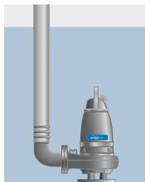
A semi-permanent free standing installation. Transportable version with pipe or hose connection.
