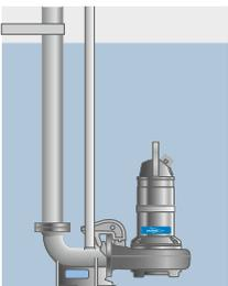
For semi-permanent wet well installations. The pump is installed with twin guide bars on a discharge connection.
