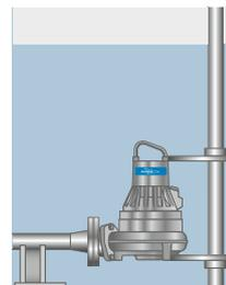
A semi-permanent installation with a swiveling guide bar for mixing and pumping. Available for 3085 and 3102.
