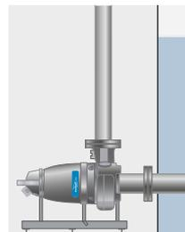
A horizontally-mounted, permanent dry well or in-line installation with flange connections for suction and discharge pipe work. Available for 3127, 3153, 3171 and 3202.
